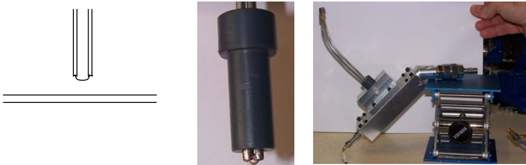
Fig. 1. Scheme and photographs of the wave probe near RF blended line.
